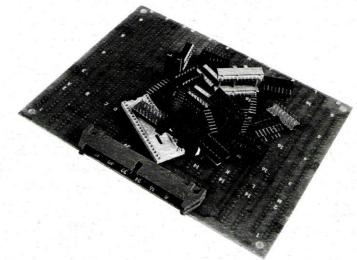
BREADBOARD with assortment of sockets for custom circuitry
