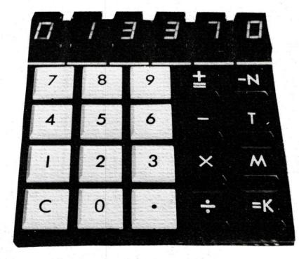
The six LED digits are driven by microcomputer output ports 015, 016, and 017. The 423's decoders display the numerals 0 through 9, and the hexadecimal numbers from A through F, thus: A, b, C, d, E, F.
